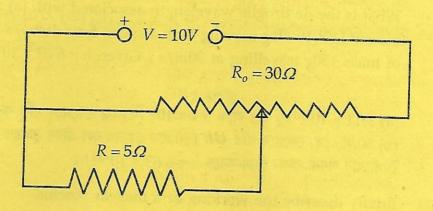
As shown in the *figure* above, a resistance of  $R = 5\Omega$  draws current from a potentiometer of total resistance  $R_o = 30\Omega$ . A voltage V = 10V is supplied to the potentiometer. What is the voltage across R when the sliding contact is in the middle of the potentiometer?
