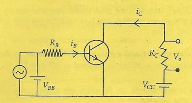
In the above circuit diagram  $V_{CC} = 8V$ ,  $V_o = 0.5V$ ,  $R_C = 800\Omega$  and  $\alpha = 0.96$ .
