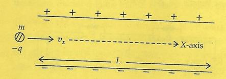
In the above diagram, a particle of mass "m" and charge (-q) initially moving along X-axis with velocity " $v_x$ " enters the region between two charged plates. The length of the plate system is "L" and uniform electric field between the plates is "E". What is the vertical deflection of the particle at the far edge of the plate?
